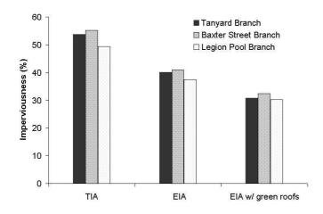
Figure 4: Total Impervious Area (TIA) and Effective Impervious Area (EIA) for three watersheds.
